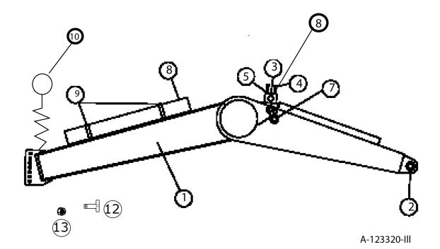
**ITEM** ΟΤΥ PART NUMBER DESCRIPTION 1 A123320 Front Section 1 2 2 2" ID x 3-1/2" OD x 3" long bronze bushing A123320-8 3 4 Trunion mount block A123293A 4 8 Bolt, 3/4" NC x 5-1/2" long, gr. 8 AFB-00039 8 3/4" lock washer 5 AFW-00002 7 2 A123320-20 Travel Lock 8 1 A125005 Accumulator 2 Mounting brackets 9 A125009 1 A125109A Hose Support 10 Trunion Bushing 11 2 A125179 7 1x5-1/2 NC Gr 8 Bolt 12 AFB-00021 13 7 AFN-0037 1" NC Locknut
