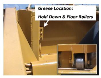
All Grease areas should be cleaned prior to greasing. Lack of grease within these pivoting areas will void your factory warranty.
