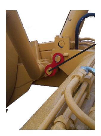
Please locate red Transport Links and remove prior to operation. Retract Lift Cylinder Circuit, Remove Safety Snap Pin, Remove link and replace into storage position as shown in figure 2. Reinstall Safety Snap Pins.
