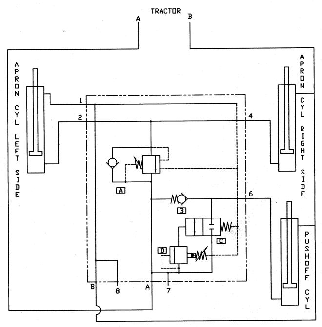
PORT 7 AND 8 ARE PRESSURE TEST PORTS #6SAE
