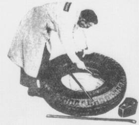
3. Lubricate last section of lower bead to facilitate mounting.
