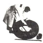
Lubricate last section of low bead to facilitate mounting.
