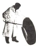
so it will not inte fere with demoun ing the secon bead. Lubricat second bead. A top of assembly in sert straight end ( tool between bea and back flange ( rim at about a 45 angle. Turn tool s it is perpendicula to rim. Pry secon bead off.
