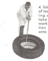
4. Using straight end of tool (with stop resting on rim flange) take small bites to work remaining section of lower bead onto rim.
