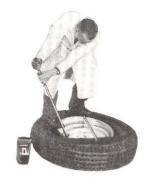
3. Stand tire and tube in vertical position with valve at top of assembly and remove valve from valve hole. Then place valve at bottom of assembly and pull out upper portion of tube so it will not inter-
