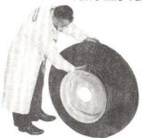
6. To get top bead in place stand on tire and force bead down as far as possible and clamp vice grip pliers on the flange. (snub side toward tire). Using spoon end of tire iron with lug side towards rim, work progressively around bead using small bites until bead slips over
