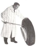
fere with demounting the second bead. Lubricate second bead. At top of assembly insert straight end of tool between bead and back flange of rim at about a 45° angle. Turn tool so it is perpendicular to rim. Pry second bead off.
