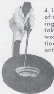
4. Using straight end of tool (with stop resting on rim flange) take small bites to work remaining section of lower bead onto rim.
