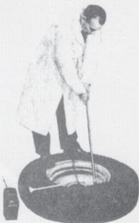
1. Remove valve core to deflate and loosen tire from bead seat of rim on both sides. Lubricate upper bead of tire thoroughly. With stops toward rim, insert spoon ends of both tools about 10 inches apart. While standing on tire to hold bead in well, pull one tool back toward center of rim.
