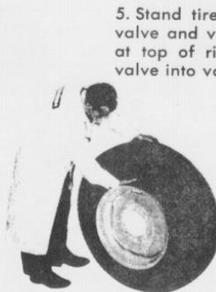
5. Stand tire up with valve and valve hole at top of rim. Insert valve into valve hole.
