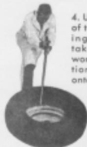
4. Using straight end of tool (with stop resting on rim flange) take small bites to work remaining section of lower bead onto rim.
