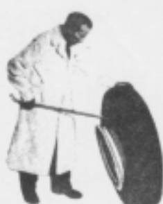
3. Stand tire and tube in vertical position with valve at top of assembly and remove valve from valve hole. Then place valve at bottom of assembly and pull out upper portion of tube so it will not interfere with demounting the second bead. Lubricate second bead. At top of assembly insert straight end of tool between bead and back flange of rim at about a 45° angle. Turn tool so it is perpendicular to rim. Pry second bead off.
